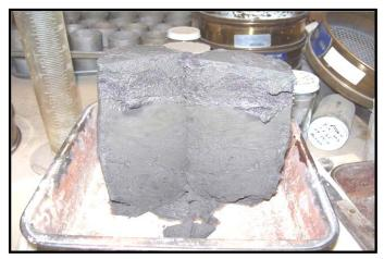
Figure 2: "Undisturbed" Fly Ash Sample: Evidence of Compression During Sampling
