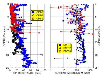
Figure 4: CPT and DMT Results
