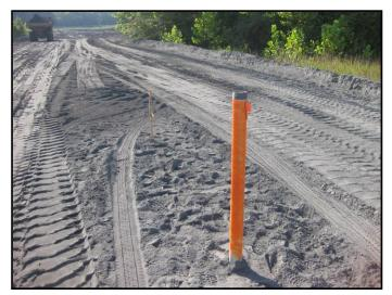
Figure 5B: Completed Settlement Plate--Long term Monitoring
